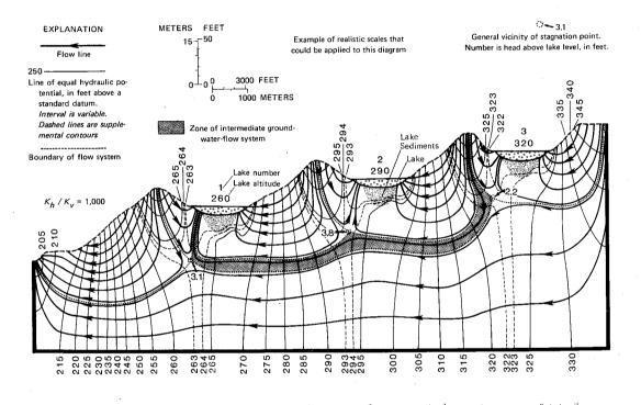
Nig.l A quali-quantitative flow net of groundwater lakes in a multiplelakes system taht does not contain aquifers. - 74
