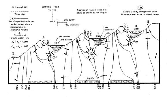
Fig. 4 Distribution of hydraulic head in the groundwater reservoir of a multiple-lakes system that has high water-table mounds and aquifers of limited extent at the base of the system.
